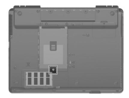
Where used: 1 captive screw that secures the hard drive to the computer
